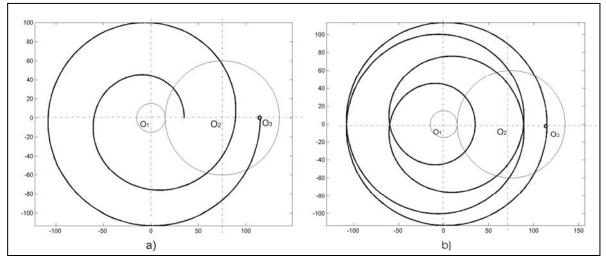
Fig.4 Trajectories of metallographic probes in the rotation plane : a) 2 rolls on the fixed circle; b) 4 rolls on the fixed circle.
