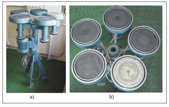
Fig. 2 Metallographic probe finishing machine
